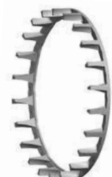
Fig. 46. Split, machined-brass, land-riding, finger-type cage.
