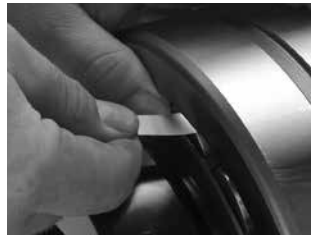
Fig. 91. Measure RIC before installation.
