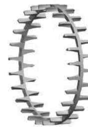
Fig. 45. One-piece, machined-brass, land-riding, finger-type cage.
