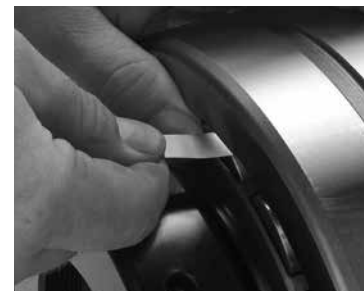
Fig. 95. Measure RIC before installation.
