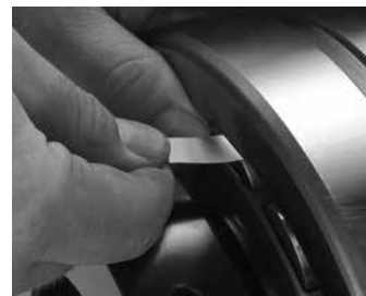
Fig. 97. Measure of RIC before installation.
