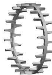
Fig. 44. One-piece, machined-brass, roller-riding, finger-type cage.
